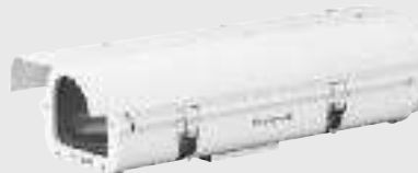
GHG-210S Indoor/Outdoor, -35°C~49°C, Inside : 110(W)x100(H)x350(D)mm, 2.8kg, Sunshield
