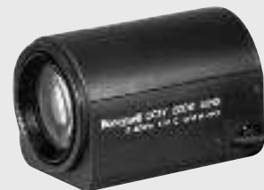
GL-A80Z10C Auto iris, Zoom lens, 8-80mm, C-mount, 1/2"
